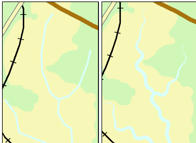
fig 3.3. Uniform stroke symbols don't portray the organic hierarchy of streams. Representation rules dynamically create sinuous curves and tapered ends to produce a natural appearance.
