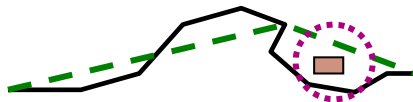
Figure 13: Simplification of line (solid to long-dashed) may cause another feature (in the circle) to be on the opposite side
