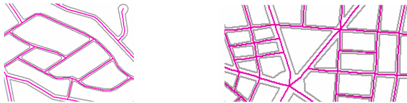
Figure 3: Examples of resulting centerlines with intersections and cul-de-sac
