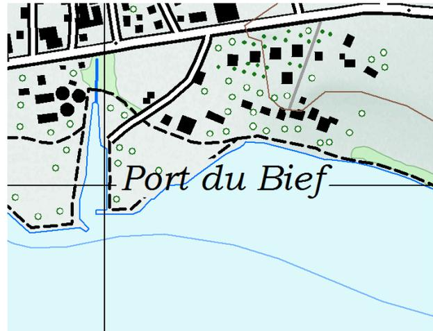
Fig. 15 - Selective Masking of Black behind Text.
