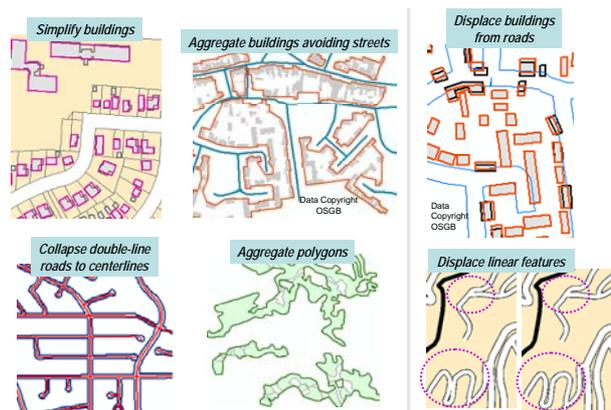
Fig. 13 - Generalization Algorithms.
