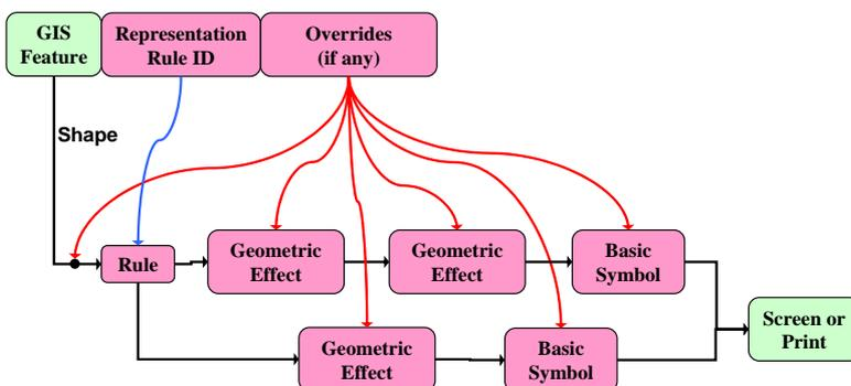
Fig. 2 - Drawing pipeline for representations with overrides.
