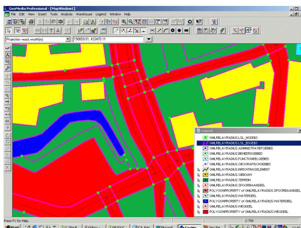
Fig. 3 - Topology - shared edges and joining nodes
